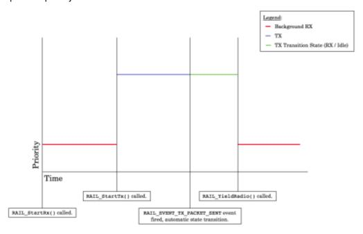
The need to actively yield the radio, and thus the RAIL\_YieldRadio() API were necessary largely due to ACK'ing.
