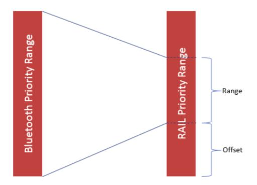
In this example the Bluetooth priority range, which itself spans from 0 to 255, is mapped to a limited portion of the shared RAIL priority space
