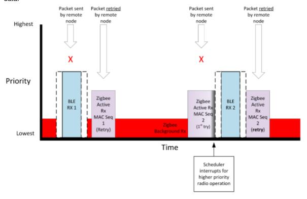
In the first case, when an IEEE 802.15.4 message is sent and the Bluetooth LE stack is utilizing the radio for an active receive the Zigbee stack will not be online to receive the message. However, the Zigbee sender of the
