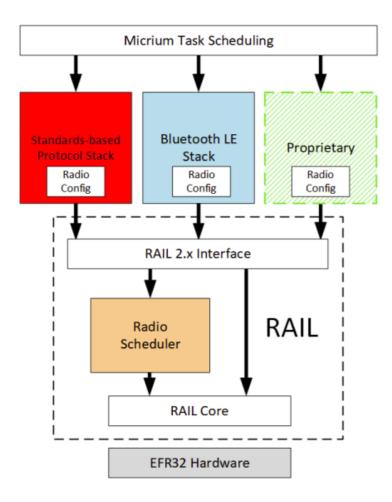
Beginning with version 2.0, RAIL requires the passing of a radio configuration handle to the RAIL API calls. This configuration describes various PHY parameters that are used by the stack
