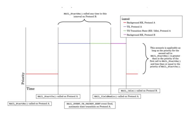
In this situation, it is important to note that RAIL\_StartRx() can be called at any time during the TX transaction. As long as its priority is less than or equal to the priority of the TX, the RX will not come into effect until the application calls \_Yield Radio() on Protocol A. When RAIL\_StartRx() is called during the TX, the RX is merely added to the queue of events to be handled.
