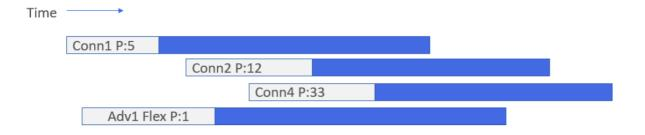
As shown below Conn1 is the first task to run as it does not overlap with any higher priority task.
