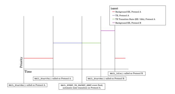
In this case, since the priority of the second RAIL\_StartRx() is higher than the priority of the call to RAIL\_StartTx(), a call to RAIL\_YieldRadio() is no longer necessary. Because the second RAIL\_StartRx() is at a higher priority, it usurps the RAIL\_StartTx() event, taking control of the radio and removing the TX event from the state. At any time during that RX on Protocol B, RAIL\_Idle() can be called to return to the RX on Protocol A, just as in the previous example.
