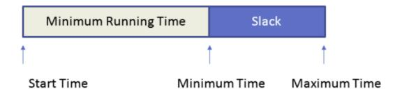
If the start time is moved the total running time is reduced respectively, that is the slack is reduced. Also priorities can be dynamically adjusted.
