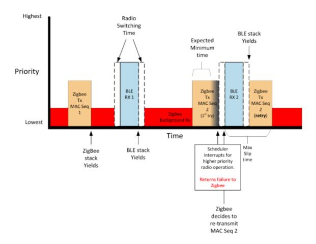
This example starts in the same way as the previous example. Zigbee and Bluetooth LE both have a radio operation that is scheduled without any collision
