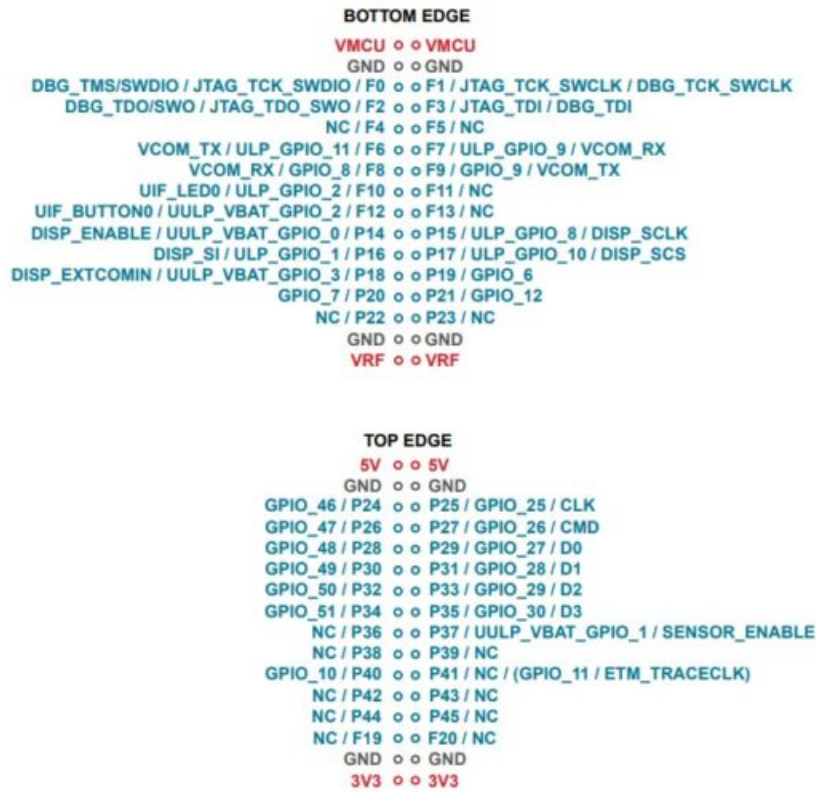
Figure 3.2. Wireless Pro Kit Mainboard (BRD4002A) Breakout Pad Pin Mapping
