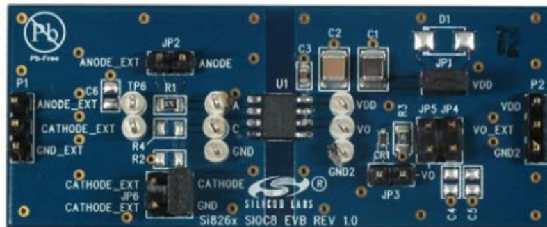
Figure 2. Si826x SOIC8 Evaluation Board Overview
