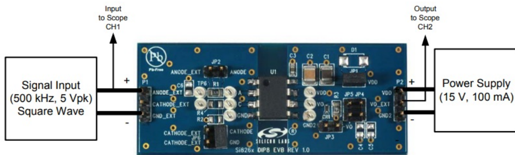
Figure 5. Summary Diagram and Test Setup
