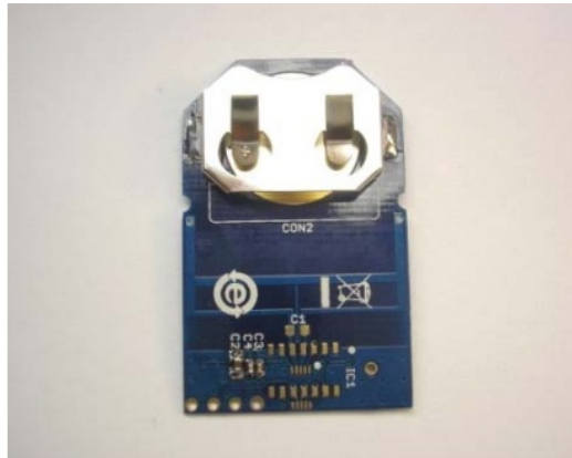
Figure 5. 4010 Key Fob Demo Board 434 MHz w/o IC (P/N 4010-KFOB-434-NF)
