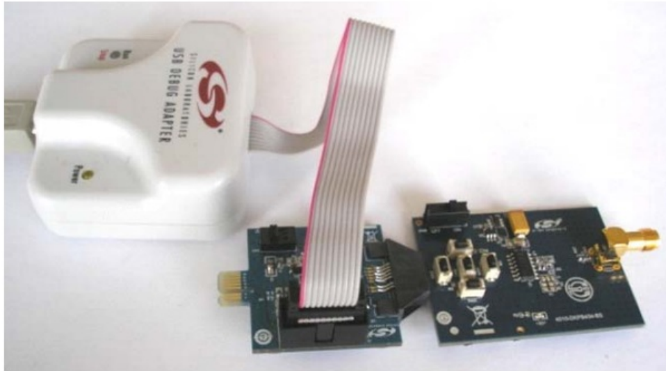
Figure 9. Target Board and Debug Adapter
