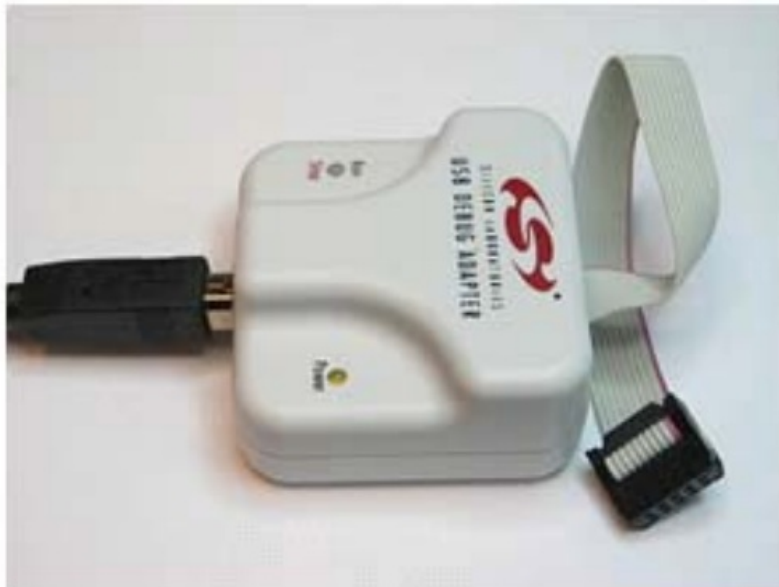
Figure 7. EC3 Debug Adapter (P/N EC3)
