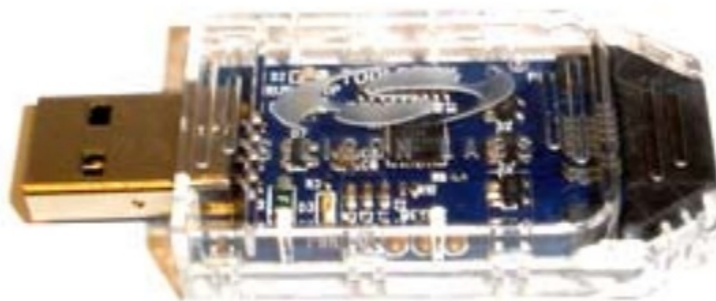
Figure 8. Toolstick Base Adapter (P/N Toolstick_BA)
