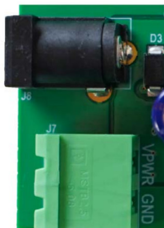
Figure 1.8. Barrel Jack with Two Terminal Power Connectors
