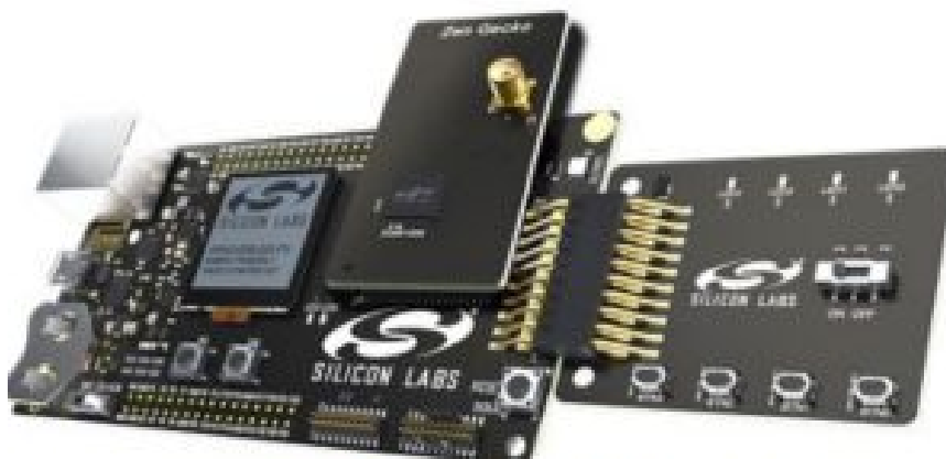
Figure 1: Main development board with Z-Wave SiP module
