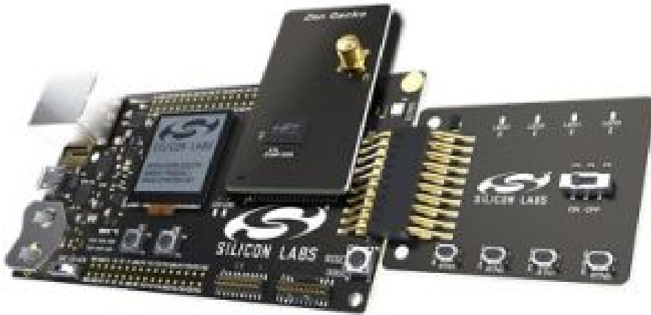
Figure 1: Main Development Board with Z-Wave SiP Module
