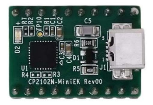
The CP2102N-MINIEK kit is designed to showcase the various features of the CP2102N USBXpress® devices. These highly-integrated USB-to-UART bridge controllers provide a simple solution for updating RS-232 designs to USB using a minimum of components and PCB space. By eliminating the need for complex firmware and driver development, the CP2102N devi-ces enable quick USB connectivity with minimal development effort.
