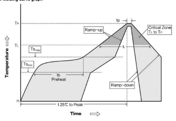
Reflow welding temperature and time
