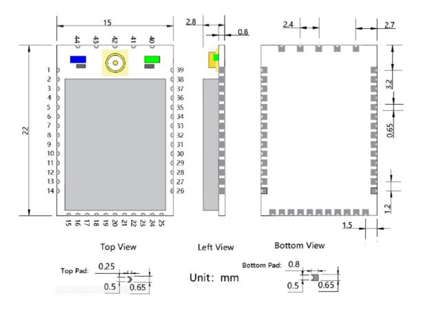
Recommended pad design: length 2\*0.8mm = 1.6mm and width 0.65mm.
