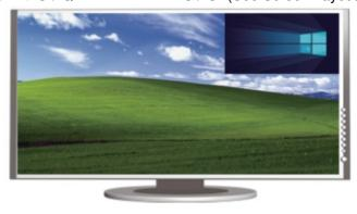
Mode 7 Features PIP Mode. Selected Computer's Content Are Showed on Display as PIP Image. Click Port Selection Button to Switch Computer. Roaming Mouse Disabled in This Mcde
