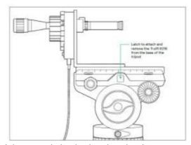
• Make sure that the Trulifi 6016 unit is securely latched to the tripod.
