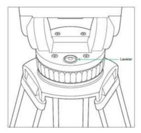
Mount the Trulifi 6016 on the tripod. Make sure that the tripod is leveled, using the leveler integrated in the tripod.
