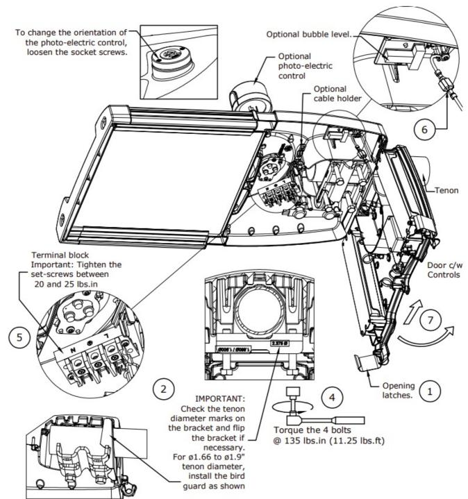
3. Disconnect power and slide the fixture onto the tenon. See table for approximate penetration. Horizontal angle can be adjusted in 2.5° steps. The optional bubble level may be used.
