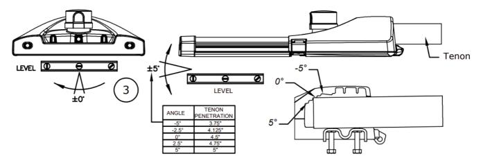
4. Evenly tighten the four bolts of the bracket.
