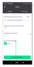
Use the DALI Power Supply (DALI PSU) feature to enable the device so it will deliver the power supply for DALI communication by itself.
