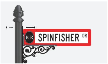
Use 5/16-18 stainless steel hex bolts, nuts & washers provided to attach scroll bracket arm to pole. Tighten securely.
