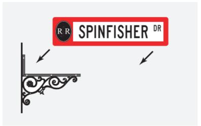
Loosen (4)  $1/4-20 \times 3/8$ " set screws. Insert street blade into channel. Be sure blade is completed seated into channel then tighten (4) 1/4-20 set screws to secure blade
