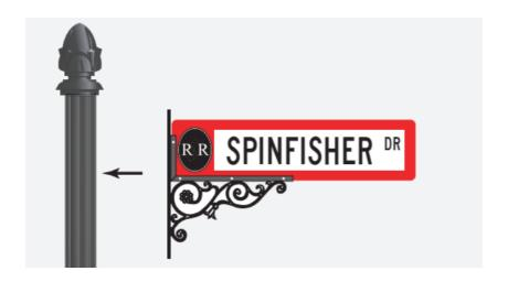
Poles may be drilled for bolt-thru attachment before or after installing pole in-ground. Use bracket to mark hole locations. Drill thru one side of pole with 3/8" drill bit. Measure to center of top hole. Mark opposite side of pole at the same height and drill holes.
