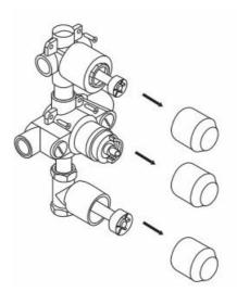
2. Slide the decorative back plate onto the valve. Ensure that the markings located above each opening on the back plate are facing up. Install the handles using the provided hex wrench.
