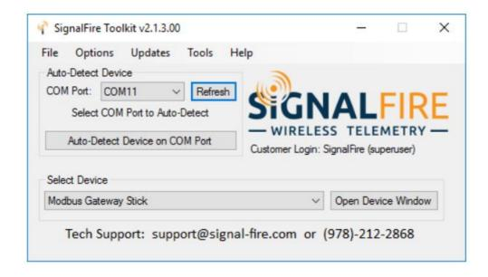
Select the COM port associated with the ModQ Flow Totalizer and click "Auto-Detect Device on COM Port." This will open the device configuration window, where all device settings can be configured.
