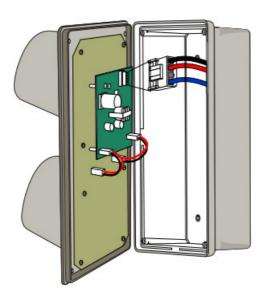
Note: Do not overtighten fasteners or distort the back panel.
