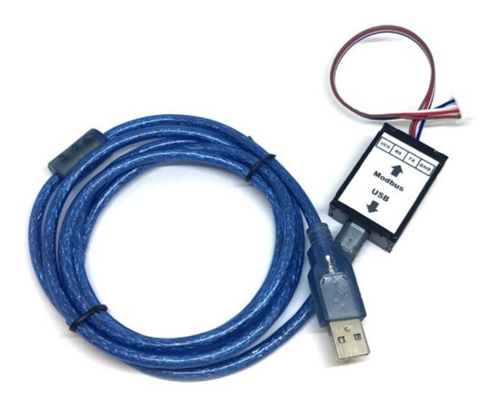
Serial port configuration on computer: 9600 baud, None parity, 1 stop bit.
