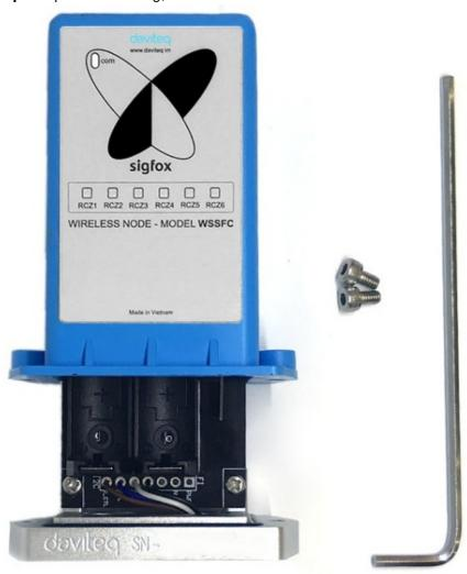
Step 4: Plug the connector to the configuration port;
