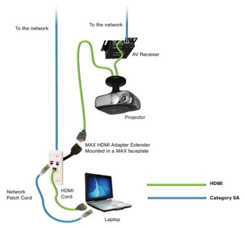
BYOD Configuration using HDMI Adapter Extender
