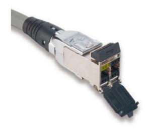
As the chosen standards-based interface for category 7A /class FA systems, TERA outlets are the highest-performing twisted-pair connectors available. When installed as part of a category 7A /class FA AV deployment, TERA offers superior delay skew performance for superior delivery of RGB video. Tera outlets feature PowerGUARD technology to prevent erosion due to arcing when a plug is unmated under remote power load.
