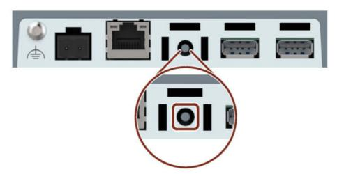
Be sure to hit the button accurately and do not slide the tool off the button.
