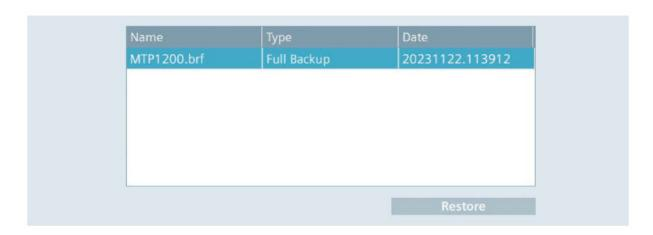
The list shows all backups that can be loaded to the HMI device.
