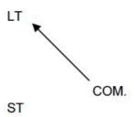
Determines timing period. LT: 30 sec -10 min, ST: 1-20 sec. Connect a jumper between common and LT or ST.
