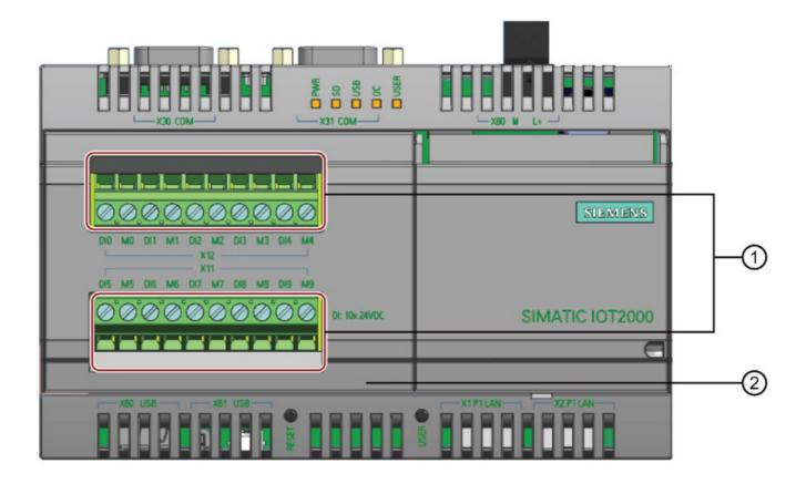
M0, M1 to M9 are all isolated by optical coupling.
