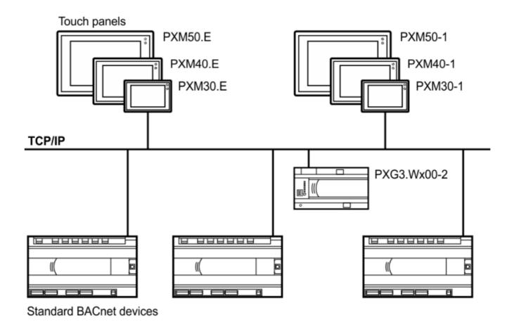
The web interfaces PXG3.W100-2 and PXG3.W200-2 are the central points of access to operate the automation level and room automation. The central point of access permits simultaneous operation on various operator units and supports
