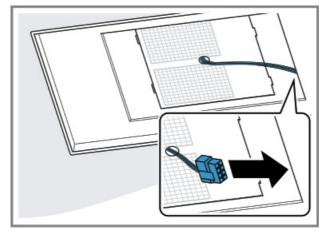
9. Press together the cable duct at the sides and attach.
