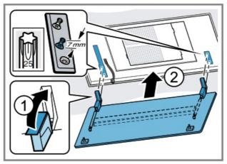
2. Mount the filter cover on the designated screws and push it backwards/forwards depending on the key hole opening into the narrow section.
