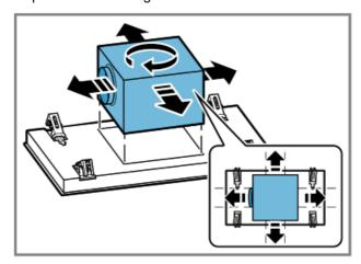
5. Push the fan box to the side and connect the appliance to the power supply.
