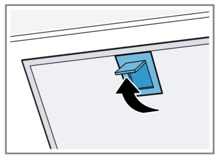
4. Remove the grease filters from the holders.
