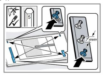
Tighten the screws one at a time so that the appliance is not wedged in the cut-out.
