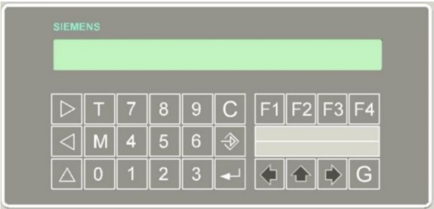
Figure 3: 2 x 40-digit LCD display with LED background lighting
