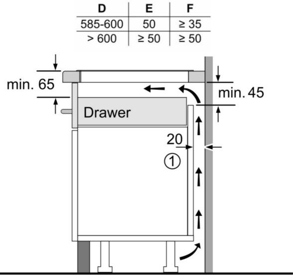
1. Ventilation gap must be present. Measurements in mm
