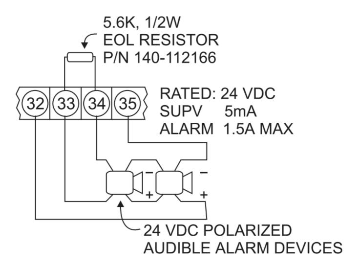
NOTE: TOTAL LINE RESISTANCE (4 WIRES) NOT TO EXCEED 36 OHMS.
