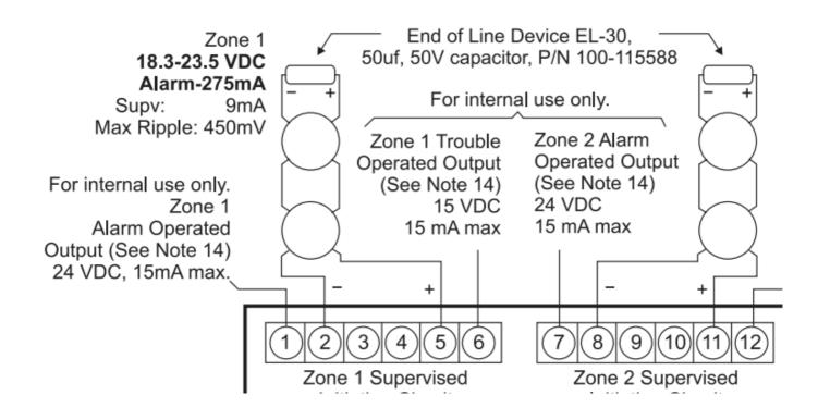
Total line resistance 36 ohms max. See Diagram A below for Class A connection. Initiating circuits are power limited per NFPA 70, National Electrical Code.
