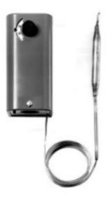
The 141 series Line Voltage Remote Bulb Thermostat is a two-position electric line voltage thermostat with a remote bulb. This device has an SPDT switch with motor ratings to 8A FLA @ 240 Vac.
