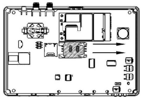
4. Lift the SIM plastic holder and replace/install the SIM card facing chip side down.
