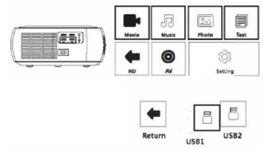
After inserting the USB flash disk, select Movie, Music, Photo, or text according to the desired content to enter the USB flash disk.
