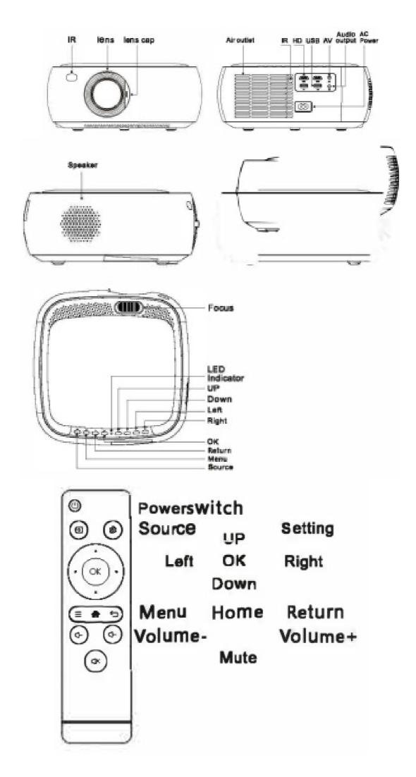
**Note:** The remote control must correspond to the Infrared or screen of the fuselage to be effective.
