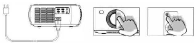
Connect the power cord to the projector, slide the lens cover to the right and the projector will start automatically. With the lens cover open, aim the remote control at the front / rear infrared window of the fuselage, and press the "U"power key to start the device.
