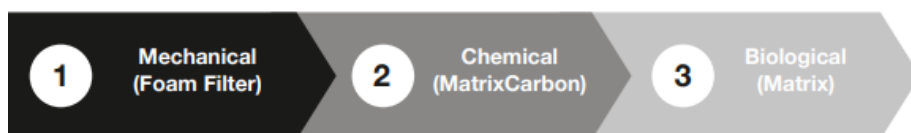
Figure 5: Layering Filtration Media (bottom to top)
