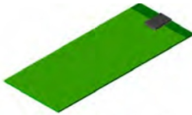
Cell phone config 1 ground plane (size: 40 x 100 mm 2 )
