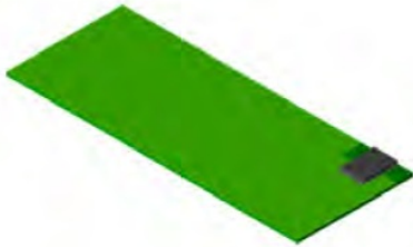
Cell phone config 2 with side ground plane (size: 40 x 100 mm 2 )
