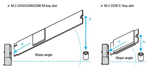
2. Install the M.2 device into the M.2 slot and secure with a screw.
