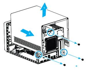
3. Unfasten the rack mount screws and remove the rack.
