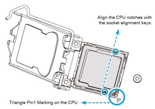
Please be aware of the CPU orientation, DO NOT force the CPU into the socket to avoid bending of pins on the socket and damage of the CPU!
