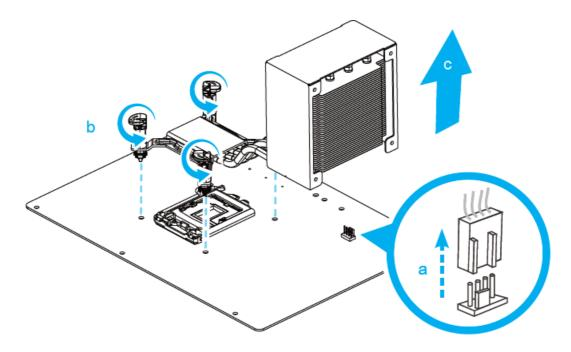
3. Remove the ICE module from the chassis and put it aside.
