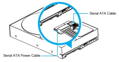
4. Connect the Serial ATA and power cables to the optical drive.
