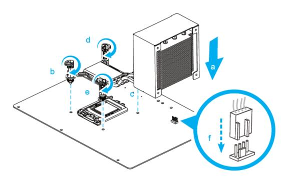
Tighten the Smart Fan to the chassis with the four thumbscrews.
