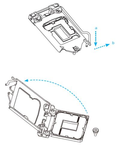
DO NOT touch the socket contacts. To protect the CPU socket, always use the protective socket cover when the CPU is not installed.
