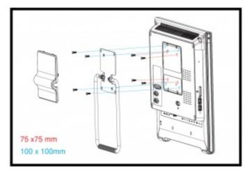
**Note**: The X50V4 can be mounted to a wall using a VESA compatible 75 x75 mm or 100 x 100mm wall/arm bracket.
