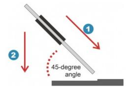
4. Carefully push down the memory module until it snaps into the locking mechanism.
