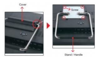
2. Unscrew four screws of the back cover and remove it.
