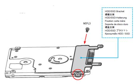
7. Connect the HDD/SSD with the appropriate cable and fasten the screws on the mainboard.
