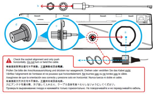
3. Please remove the connector of the internal antenna. To avoid a short circuit, please ensure that insulation tape is wrapped around the antenna connector before putting it aside. Now connect the WLAN antenna cable to the I-PEX connector and affix with adhesive tape, as shown.
