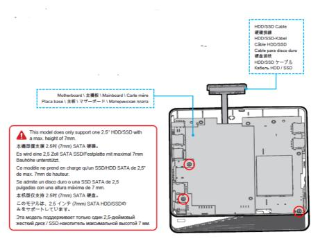
6. Place the HDD/SSD in the bracket and secure with two screws.
