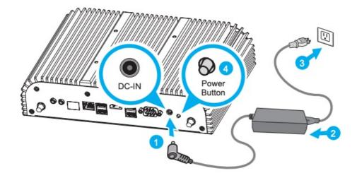
CAUTION: Do not use inferior extension cords as this may result in damage to your Box-PC. The Box-PC comes with its own AC adapter. Do not use a different adapter to power the Box-PC and other electrical devices.
