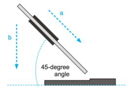
5. Repeat the above steps to install an additional memory module, if required.
