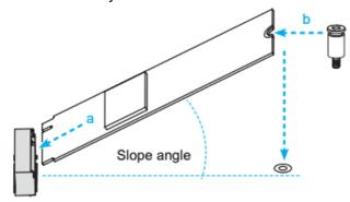
2. Install the M.2 device into the M.2 slot and secure with the screw.
