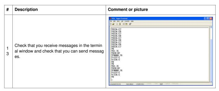
This section describes how to test the ECA commands using a second PC and Microsoft Terminal program.
