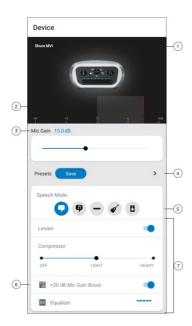
**Notifications** The top row displays which device is connected. A red flashing dot next to the name let you know whether recording is active. The charms show which advanced features are on. Tap the headphone icon to access direct monitoring control. Tap the lock to lock or unlock the settings.
