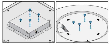
5. Lift the microphone and align the thumbscrews with the holes in the VESA bracket. Tighten the thumbscrews to secure
