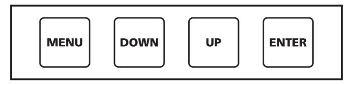
• MENU: switch through setup menu. Press 3s switch to advanced interface
