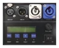
LCD information display area, showing operate menu and working status of machine.
