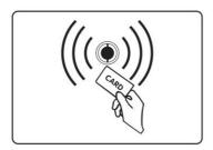
RFID card comes together with HC8200. It is a safety design, allows machine to identify the parameter and types of consumable. Please note that granules RFID card can increase the single machine specific working time. The card is disposable, can only use once.
