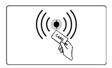
RFID card come with consumable HC8600 bags, swiping card to identify parameters and types of granules. The RFID card is disposable, one card can only use one time. Each card can increase single machine 20min working time, the maximum recharge time for SPARKULAR ® II is 30min
