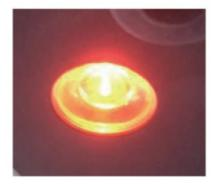
Off Sparking or Not in preheating Quick Flashing Preheating Long on Preheated Slow Flashing Error warning
