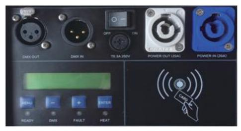
LCD information display area, showing operate menu and working status of the machine.
