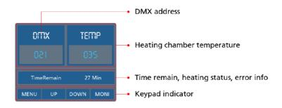
Background color of DMX area: red means DMX connected. Background color of TEMP area: red means heating chamber temp. reached setting temp. machine is ready for firing. Indicator light status on power switch: flash means machine is heating up, long on means temp. reached setting temp.
