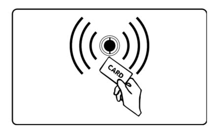
RFID card come with consumable HC8200 bags, swiping card to identify parameters and types of granules. The RFID card is disposable, one card can only use one time. Each card can increase single machine 20min working time, the maximum recharge time for SPARKULAR ® II is 30min
