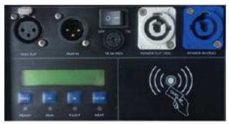
LCD information display area, showing operate menu and working status of machine.
