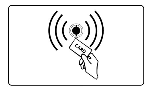
Composite Ti with RFID card, swiping cards used to identify parameters and types of granules. The RFID card is disposable, one card can only use one time.
