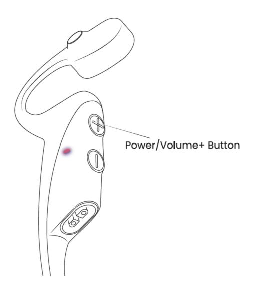
1. Start with OpenComm turned off. Press and hold the Volume+ button until the LED Indicator flashes red and blue.
